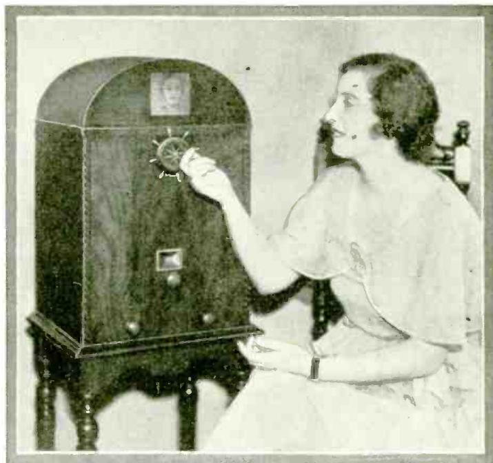
Left: Miss Speed Freeman adjusting the television tuner control on latest model, vertical cabinet receiver. This receiver comprises two distinct radio sets, one tuning in the "image" signal, and the other the "voice" signal, which is heard on a loud speaker placed at the bottom of the cabinet. The new Garner high-intensity neon tube, throws an enlarged image on the screen at the top of the cabinet.
